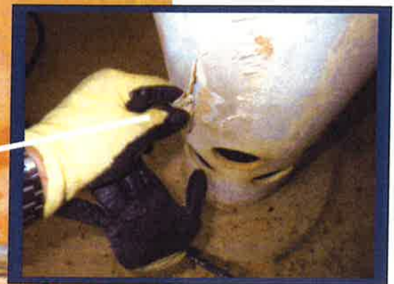
Image #6. May 3. The lower area of the fill pipe where failed coating was noted, although there isn't any significant corrosion visible.
