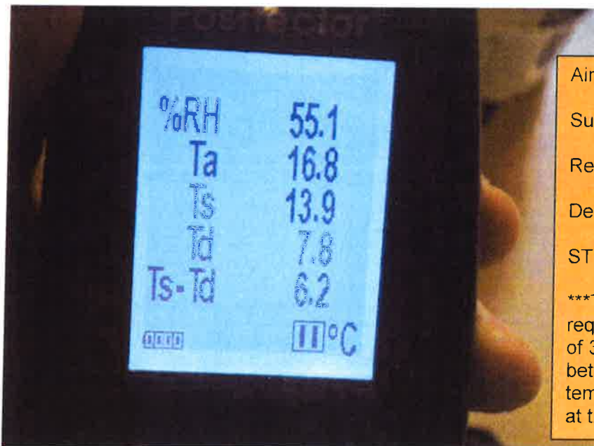
Image #16. May 5th. All Environmental Measurements taken from various locations within the vessel yielded levels above the coating suppliers requirements.
